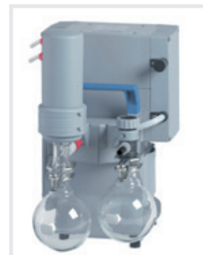
Vacuubrand MD 4C NT AK+EK (3,4m³/h, vide atteignable 1,5 mbar)
